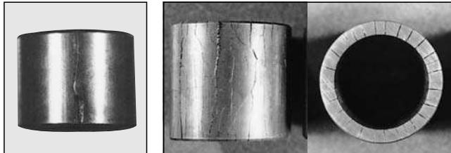
When a roller fractures during operation, typically vertical splitting occurs as shown in the photo, and in general, pitch marks of fatigue extend from the inside of the roller and cause splitting. If splitting occurs all at once due to a large tension, the cause can be identified easily since the split faces are not polished. If tension is excessive, the rollers are forcefully pressed against the tooth faces of sprockets, and a roller end may be cracked and deformed.
