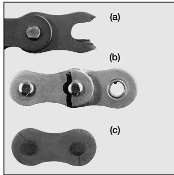
(b). A significant feature of fatigue fracture is that a crack occurs in the direction almost perpendicular to the pitch line (center line between both pins). In the case of hydrogen embrittlement by an acid, the crack mostly occurs in the direction as shown in (c), and the cut ends are flat, while the area around the cut ends may be decolored due to erosion by the acid.
